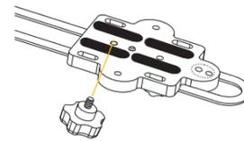
6. Attach the camera to the baseplate using the camera mounting screw. Tighten securely.
