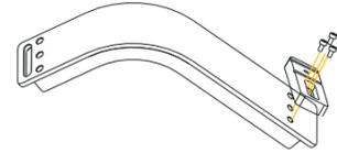
2. Attach the shoulder mount frame to the shoulder pad using the shoulder mount frame mounting plate and the included shoulder mount frame mounting plate screw. With the screw in place, you can adjust the vertical height of the rig by loosening the screw slightly and moving the shoulder mount frame up or down until it's at desired height. Then tighten the mounting screw securely. Do not overtighten.
