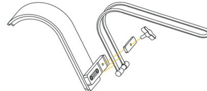
3. Attach the camera baseplate to the shoulder mount frame using the baseplate mounting plate and the baseplate mounting plate screw. After the baseplate is mounted to the shoulder mount frame, you can adjust the baseplate by loosening the screw and sliding the baseplate forwards or back. When the baseplate is in the correct position, tighten the mounting screw securely. Do not overtighten.
