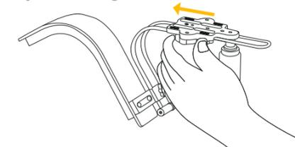
8. To adjust the vertical position of the camera, loosen the shoulder mount frame mounting plate screw and slide the shoulder mount frame up or down to the desired position. Tighten the screw securely. Do not overtighten.
