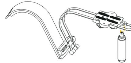
5. Screw the camera mounting screw into the camera baseplate using one of the holes provided.
