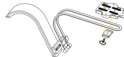
4. Mount the hand grip to the shoulder mount frame by screwing the end of the hand grip into the hole provided at the end of the camera baseplate. Align the hand grip correctly to the hole, which is angled slightly. Tighten the hand grip securely.
