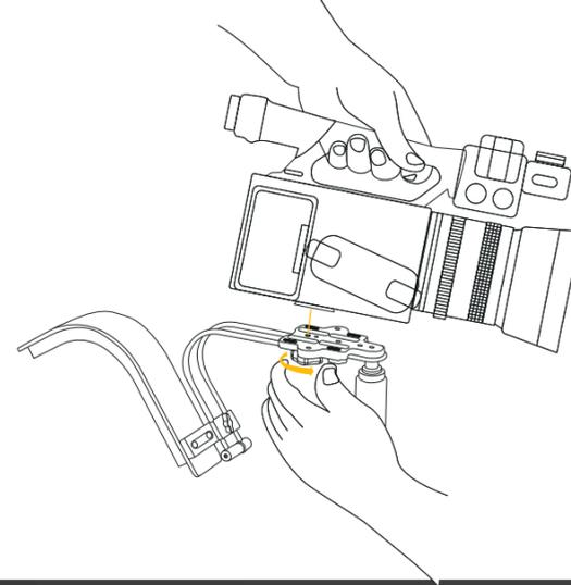
7. Adjust the distance of the camera from your eye by loosening the baseplate mounting screw slightly and sliding the camera forward or back to the desired position. Tighten the screw securely. Do not overtighten.
